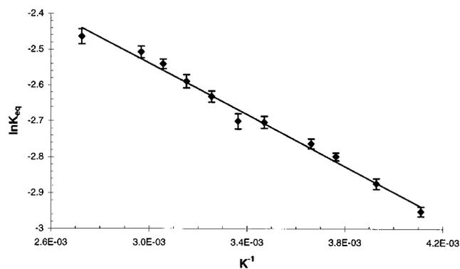
**Figure 1.** Plot of  $\ln K_{eq}$  vs  $1/T$  for the equilibrium defined in Scheme 4 for trimethylsilyl ester **7a** ( $R^2 = 0.988$ ). From the slope,  $\Delta H^\circ = 3.0 \pm 0.1$  kJ mol<sup>-1</sup>. From the intercept,  $\Delta S^\circ = -12.1 \pm 0.4$  J mol<sup>-1</sup> K<sup>-1</sup>.
