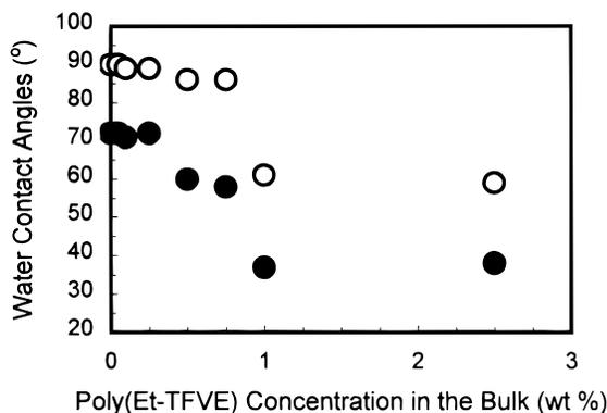
**Figure 8.** Dynamic (○) advancing and (●) receding water contact angles of PS/poly(Et-TFVE) blend film surfaces cast from *toluene* decrease with increasing poly(Et-TFVE) bulk content.
