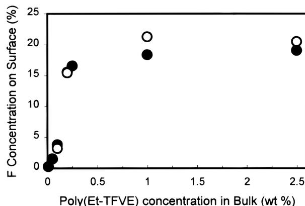
**Figure 2.** Surface fluorine atomic concentration increased with poly(Et-TFVE) bulk content at both XPS takeoff angles of (●) 15° and (○) 90°.
