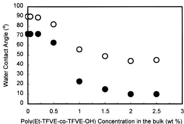
**Figure 9.** Dynamic (○) advancing and (●) receding water contact angles of PS/poly(Et-TFVE-*co*-TFVE-OH) blend film surfaces decrease with increasing poly(Et-TFVE-*co*-TFVE-OH) bulk content.
