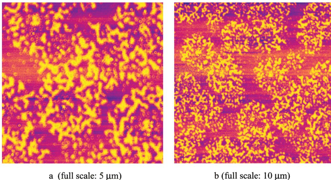
**Figure 7.** AFM images of poly(Et-TFVE) aggregates on mica surface at (a) high magnification (field width =  $5 \mu\text{m}$ ) and (b) low magnification (field width =  $10 \mu\text{m}$ ).
