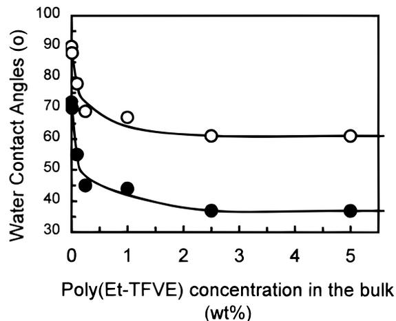
**Figure 5.** Dynamic (○) advancing and (●) receding water contact angles of PS/poly(Et-TFVE) blend film surfaces cast from *chloroform* decrease with increasing poly(Et-TFVE) bulk content.
