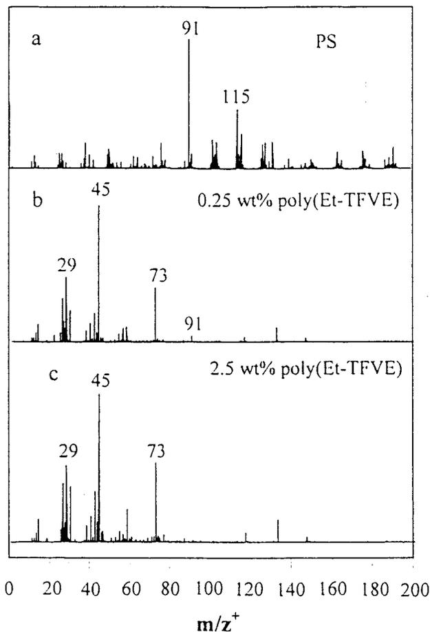
**Figure 4.** ToF-SIMS spectra of (a) PS, (b) PS/PTFVE blend having 0.25 wt % poly(Et-TFVE) in the bulk, and (c) PS/PTFVE blend having 2.5 wt % poly(Et-TFVE) in the bulk.
