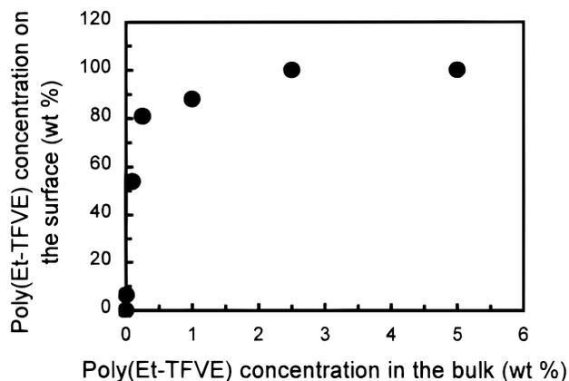
**Figure 6.** Surface composition of PS/poly(Et-TFVE) blends were estimated by the Cassie equation: poly(Et-TFVE) saturated the surface as poly(Et-TFVE) content in the bulk increased.
