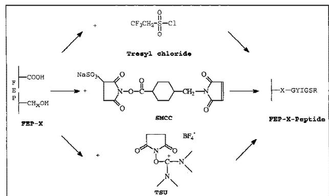
**Figure 2.** Three coupling agents (tresyl chloride, SMCC, and TSU) were used to couple the GYIGSR peptide to functionalized FEP (FEP-X) film surfaces, yielding FEP-X-peptide.
