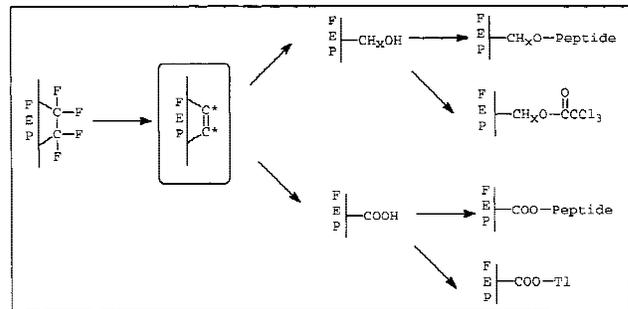
**Figure 1.** Poly(tetrafluoroethylene-*co*-hexafluoropropylene) (FEP) film samples were surface modified to either hydroxyl or carboxylic acid groups which were in turn either labeled with trichloroacetyl chloride or thallous ethoxide, respectively, or coupled with cell-adhesive peptides.
