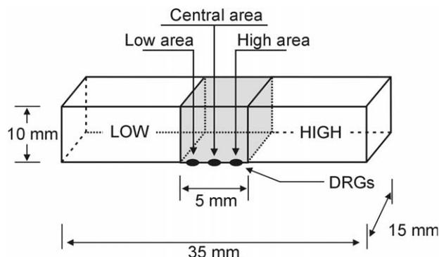
**Fig. 1.** Compartmentalized diffusion chamber for cell culture. Shaded area (agarose membrane) separates two equivalent compartments, each of which contains a constant, yet different, concentration of NGF or combinations of neurotrophins (i.e. NGF/NT-3 and NGF/BDNF). DRGs are plated beneath the agarose membrane, and cellular responses are observed under three different areas.
