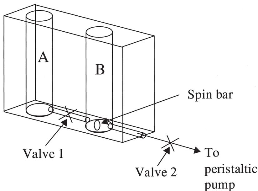
**FIG. 1.** Schematic of a gradient maker used to create gradients of NGF and NT-3 in p(HEMA) scaffolds. The monomer formulation is added to both chambers A and B and the conduit that connects the two. For neurotrophin gradients, the neurotrophin is added to chamber A only, with the concentration of neurotrophin added impacting the resultant gradient.
