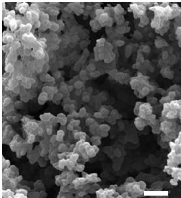
**FIG. 3.** Representative scanning electron micrograph image of a p(HEMA) scaffold used in this study. scale bar, 5  $\mu\text{m}$
