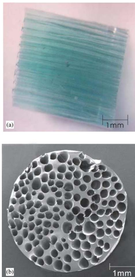
Fig. 1. A transparent P(HEMA-*co*-AEMA-1%) scaffold: (a) stained with 0.4 % Giemsa methanol and viewed by a longitudinal cross-section by light microscopy and (b) a horizontal cross-section of a scaffold of the same scaffold viewed by SEM had a mean and standard deviation of  $132 \pm 5$  channels.
