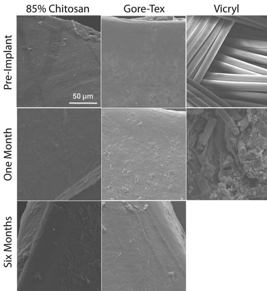
**FIGURE 3.** Scanning electron micrographs of intrathecal chitosan (DD = 85%), Gore-Tex, and vicryl sheets prior to implant and 1 and 6 months after implant. Chitosan and Gore-Tex show no significant signs of degradation. There was no vicryl sheet remaining at 6 months. All images are shown at the same magnification.
