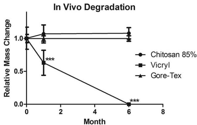
**FIGURE 2.** Measurement of weight change of implants removed after 1 and 6 months. Vicryl is the only material that exhibited degradation as assessed by weight loss ( $n = 4$ , mean  $\pm$  standard deviation, \*\*\* $p < 0.001$ ).
