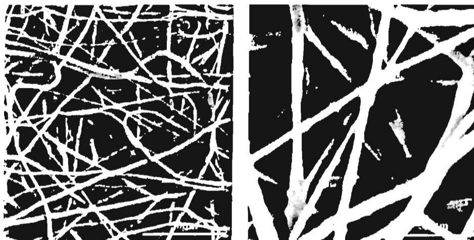
Figure 1. SEM images of the electrospun PCL scaffolds at different magnifications. The average fibre size in the PCL scaffolds is 750 \pm 100 nm (mean \pm standard deviation, n = 3 ).
